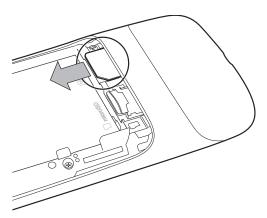
Insert the SIM card by aligning it (notch to the top left and gold contacts down) and then sliding it into its slot.
