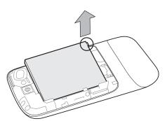
▶ Slide the battery into place by aligning the gold contacts on the phone and the battery and then gently pressing the battery into place.
