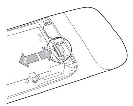
▶ Insert the microSD card by aligning it and then sliding it into its slot.
