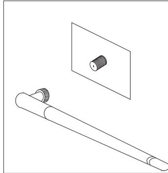
**WiFi antenna connector** — To connect the computer to a wireless network. Screw the WiFi antenna on the WiFi card connector if the model you purchased is equipped with the WiFi card.
