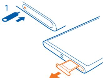
2. Make sure the contact area is face up, and put the card in the holder.
