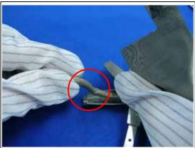
Release the cable from cover hinge.
