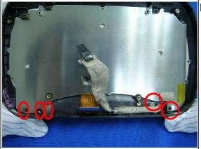
Release 5 screws on keypad bezel.
