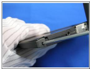
Insert screw driver into the hole and press to release the hook.
