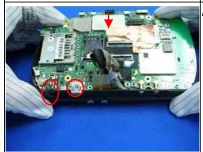
Assemble M/B from connector side.
