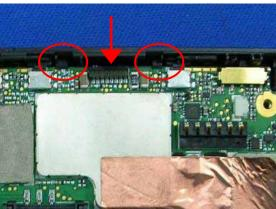
Assemble M/B into 2 hooks.
