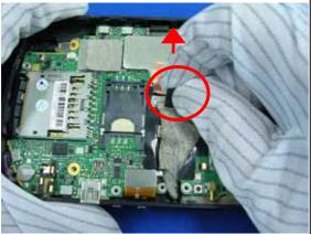
Pull out LCD coaxial cable (Display).
