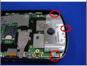
Assemble the antenna and fasten 3 screws to fix it.
