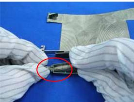
Assemble LCD cable into cover hinge.
