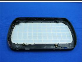
Assemble keypad into bezel.
