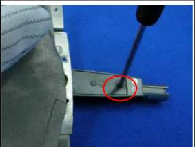
Fasten one screw to fix LCD cable with cover hinge.
