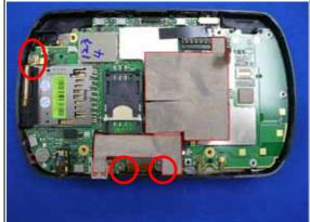
Remove 2 conducting tapes and unfasten 3 screws.
