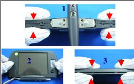
Assemble LCD housing with bezel.
