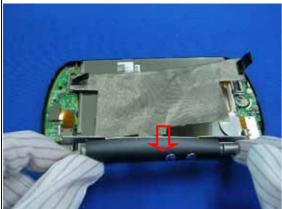
Assemble LCD coaxial cable module with LCD bezel.
