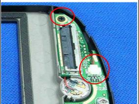
Assemble lower cover board and fasten one screw to fix it.
