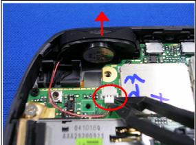
Release speaker's connector, then remove the left speaker.
