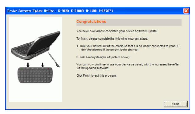
5. Cold boot the device - Press & Hold two "-"key, and use stylus to reset device.
