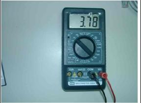
b. The battery voltage will appear on the multi-meter,
