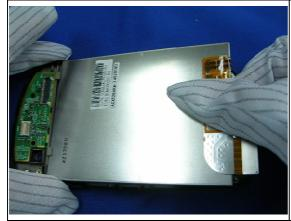
Assemble LCD into bezel.
