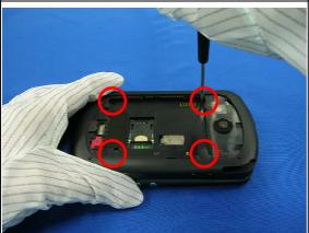
Assemble keypad housing with bezel, and fasten 4 screws on housing.
