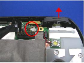
Peel off the Mylar, release speaker's connector, then remove the right speaker.
