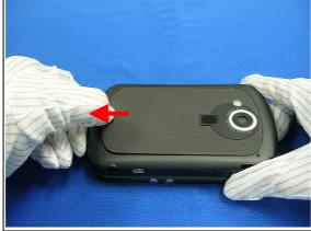
Unlock battery cover and remove it.
