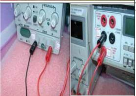
4. Connect cable of fixture( C ) to negative polarity of power supply (A) and current meter (B)
