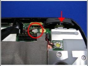
Connect the cable and assemble the right speaker.
