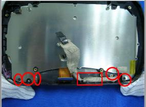
Fix LCD coaxial cable on Keypad bezel properly, and fasten 5 screws on bezel.
