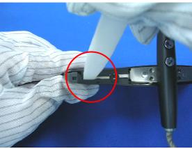
Insert plastic stick into the left side gap between LCD housing and bezel.
