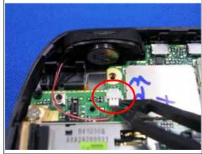
Connect the cable and assemble the left speaker.
