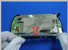
Remove LCD coaxial cable module.
