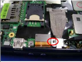
Assemble LCD coaxial cable cover and fasten one screw to fix it.
