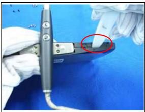
Insert plastic stick into the right side gap between LCD housing and bezel.
