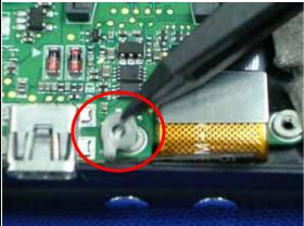
Assemble WiFi antenna and fasten one screw to fix it.
