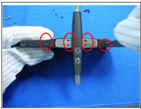
Fasten 6 screws on LCD module.
