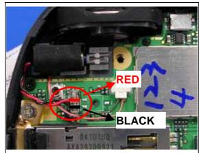
Connect the cable and assemble the vibrator.
