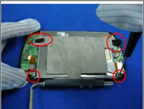
Connect cable with upper cover board and lower cover board.
