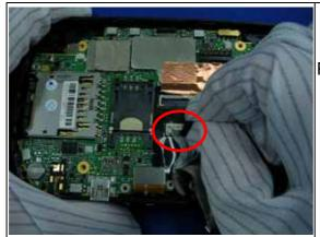
Pull out LCD coaxial cable (functional).
