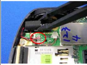
Release the vibrator connector, then remove the vibrator.
