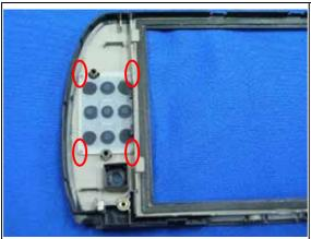
Assemble navigation button to LCD bezel.
