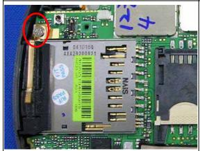
Stick on BT antenna and fasten one screw to fix it.
