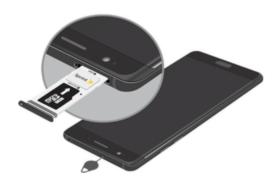
3. Slide the SIM card/Memory card tray back into the slot.
