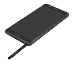
**Caution**: When you insert the S Pen into the slot, insert the S Pen's tip first. Failure to do so can cause the S Pen to become stuck. Forcefully detaching the S Pen from the slot may cause damage to the S Pen and your device.
