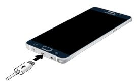
Connect the USB cable to the charging head, and then plug the charging head into a standard outlet. When charging is complete, unplug the charging head from the outlet and remove the USB cable from the device.
