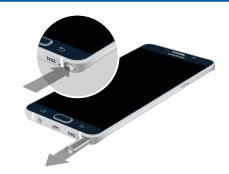
**Warning**: Be sure to insert your S Pen with the nib pointed inward. Inserting the S Pen the wrong way can cause it to become stuck and can damage the pen and your phone.
