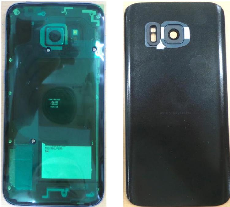
Before re-assembling, **the outside tape & inside tape** should be changed.
