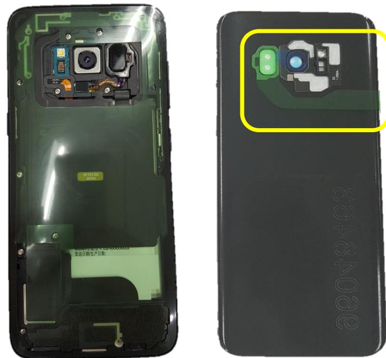
Before re-assembling, **the outside tape & inside tape & finger print sensor tape** should be changed.
