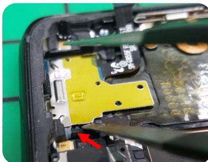
**Sensor FPCB :** Gently insert top-round tweezers to the left hole for disassembly and lift it up softly.
