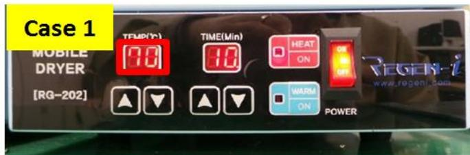
Put the device into Mobile Dryer.(70°C/10mins)
