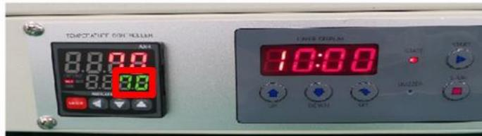
Put the device in to HOT PLATE.(70°C/10mins)
