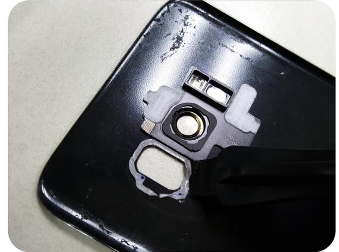
❖ Do not push the finger print sensor from the backside to detach the finger print sensor.
